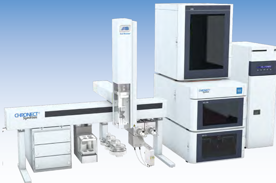
FIG. 1: CHRONECT Symbiosis Advanced , Sampler shown with options: 2nd valve, Peltier Stacks 6DW, vortexer solvent module
