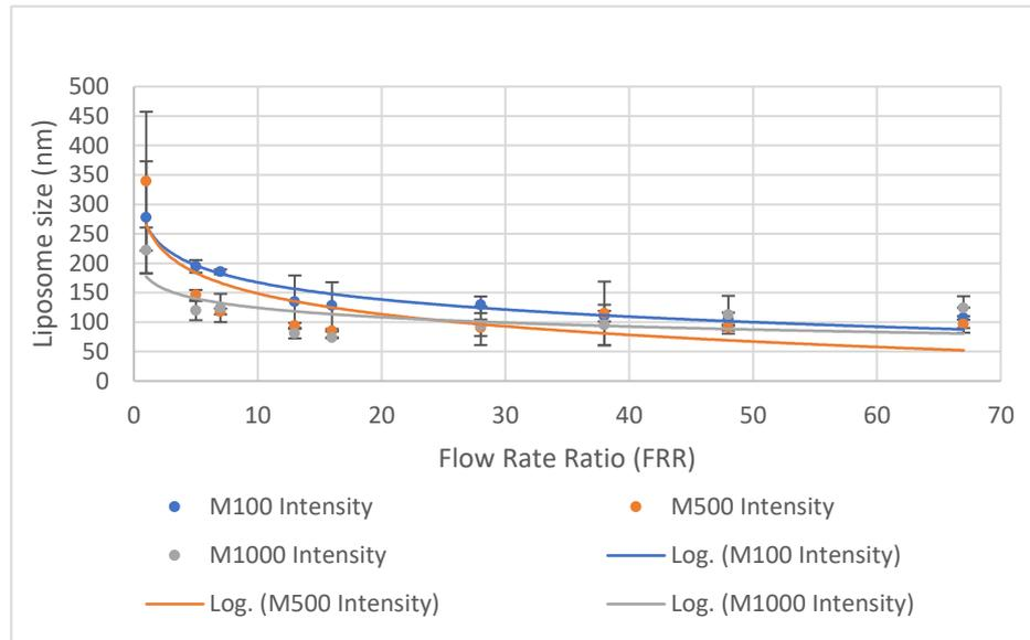
Figure 11 Peak intensity of liposome nanoparticles produced using a Micromixer chip at different FRR with TFR of 100 (M100), 500 (M500) and 1000 (M1000)  $\mu\text{l}/\text{min}$ . Average of 3 set of measurements.
