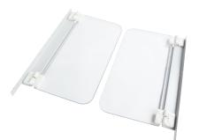
Sash Opening Reduction Wing Kits. Wings reduce sash opening area to increase face velocity to 100 FPM at the 16" sash stop position. Hinged with detents to maintain open position for loading and closed position for normal operation. For use with Echo Benchtop Filtered Fume Hoods. Shipping weight 5 lbs. (2 kg)
