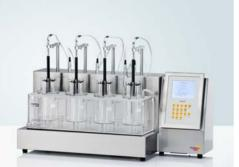
PTZ AUTO EZ Fully-Automated Disintegration Testers
