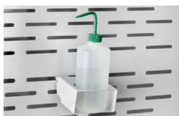
**3927700—Bottle Holder.** For use with Protector XVS Ventilation Stations. Attaches to the rear baffle perforations to hold a squirt bottle or other round container. Powder-coated steel. 3" diameter opening. Shipping weight 1.0 lb. (0.5 kg)
