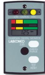
**Guardian™ Digital Airflow Monitor Kits.** LCD displays average face velocity. Audible/visual alarm alerts user to low or high face velocity. For installation in a factory-prepared cutout on upper portion of right side fixture panel. Shipping weight 6.0 lbs. (2.7 kg)
