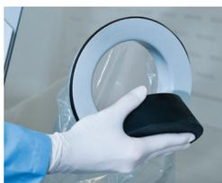
**5248300—Waste Chute Stopper.** For use with 5', 6' and 8' Protector XVS Ventilation Stations, 35.5" deep, with waste chute. When waste chute is not in use, the stopper helps prevents contaminants from escaping the enclosure through the side wall. Solid rubber. 5" diameter. Shipping weight 1.0 lb. (0.5 kg)
