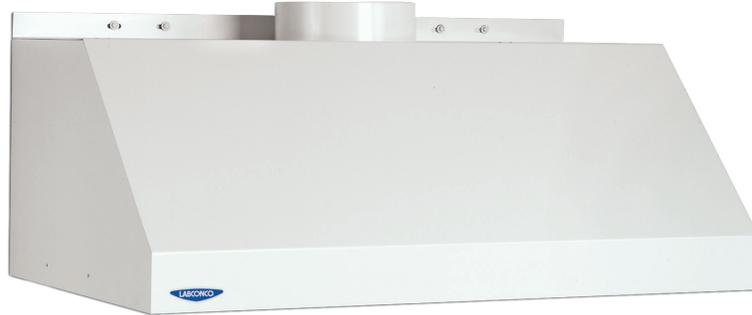
The Canopy Hood is specifically **designed to vent non-toxic materials such as heat, steam and odors** from large or bulky apparatus such as ovens, steam baths and autoclaves. The hood may be installed on a wall or suspended from the ceiling for peninsular and corner locations. **For most efficient performance, the hood should be installed no more than 12" above the equipment to be ventilated.** Coupled with a blower and ductwork, the Canopy Hood can operate at a wide range of exhaust rates.
