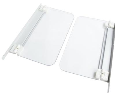
**Sash Opening Reduction Wing Kits.** Wings reduce sash opening area to increase face velocity to 100 FPM at the 16" sash stop position. Hinged with detents to maintain open position for loading and closed position for normal operation. For use with Echo Benchtop Filtered Fume Hoods. Shipping weight 5 lbs. (2 kg)
