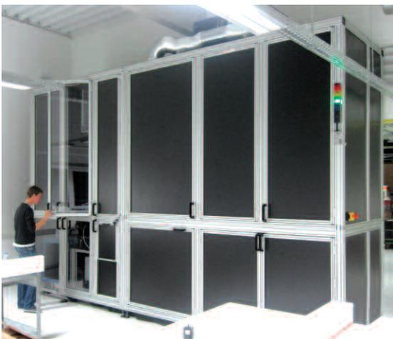
This BOD robot enclosure is a real example of full laboratory automation. It fully preps the samples including filtration, pH adjustment, dilution. BOD analysis is then done, adding ATU, stirring and reading. The system transports trays to and from the temperature controlled incubation chamber. It also features automatic storage, washing and drying of 1440 BOD bottles.
